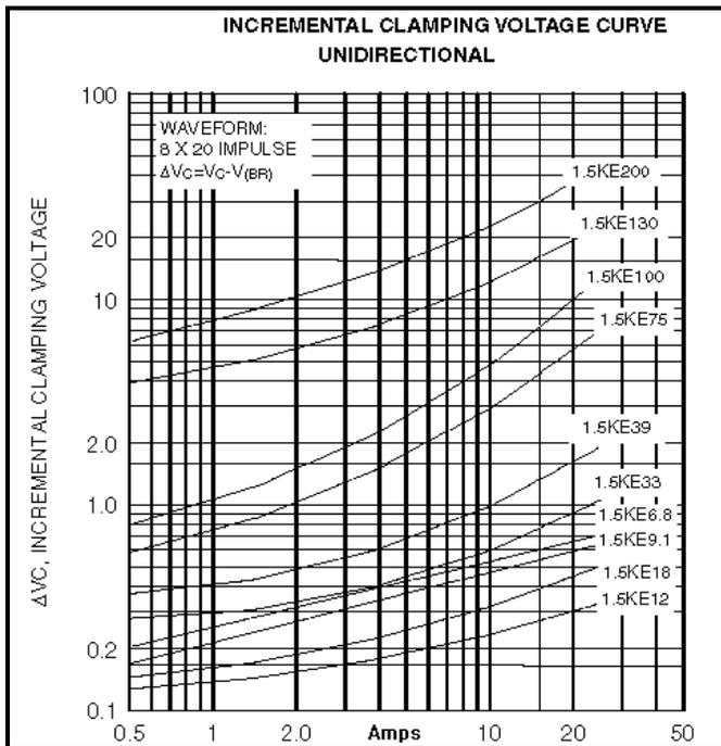
Figure 2. Incremental Voltage Values for 1.5KW Transorbs.
