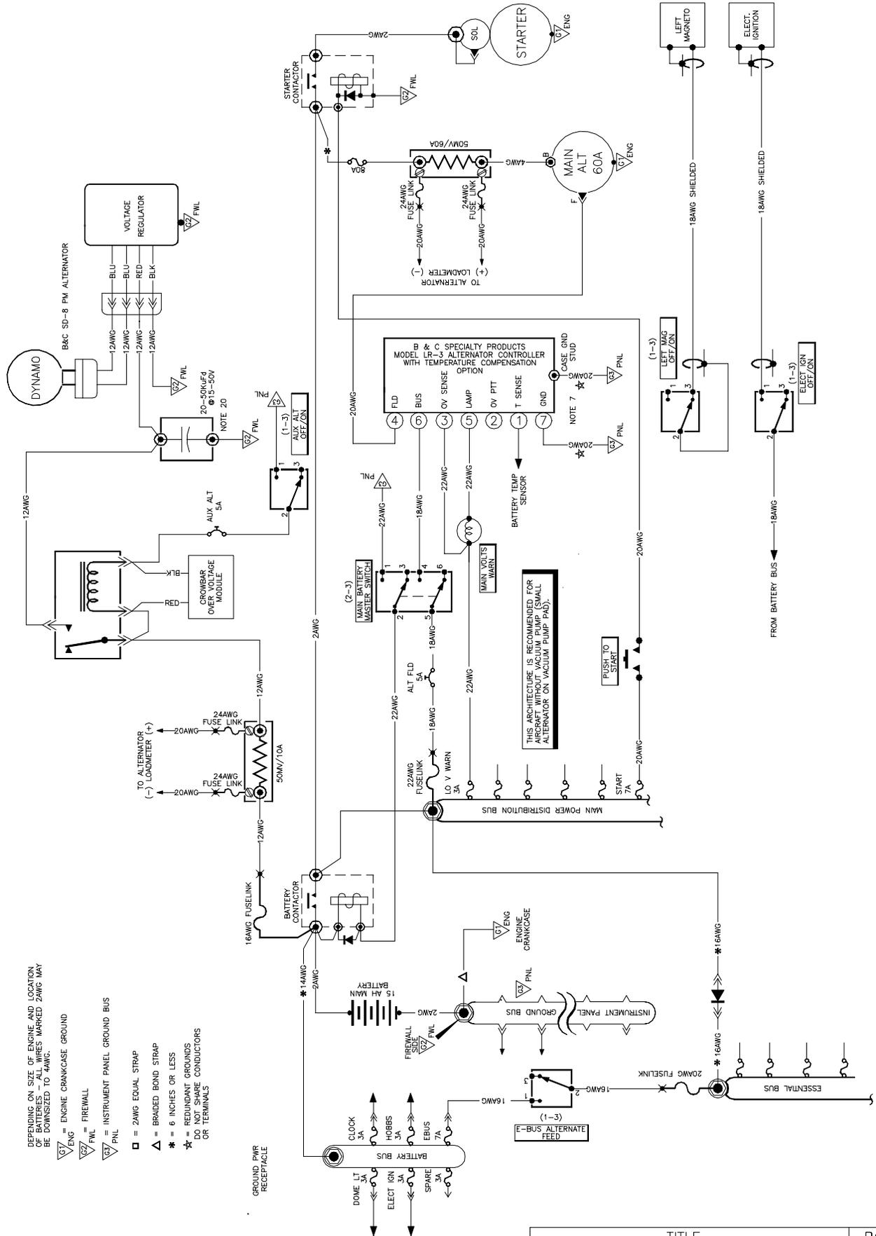
DEPENDENT ON SIZE OF ENGINE AND LOCATION OF BATTERIES - ALL WIRES MARKED 2AWG MAY BE DOWNSIZED TO 4AWG.
