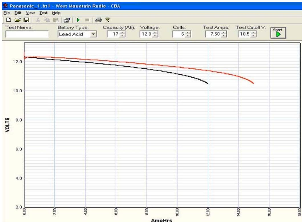
First at 4A (48 watts) and then at 7.5 amps (92 watts). Curves for these two tests are shown here.
