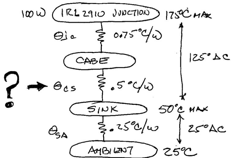
The thermal model has marginal headroom for ambient and production variables. How about hot day ambient? And in particular, are there
