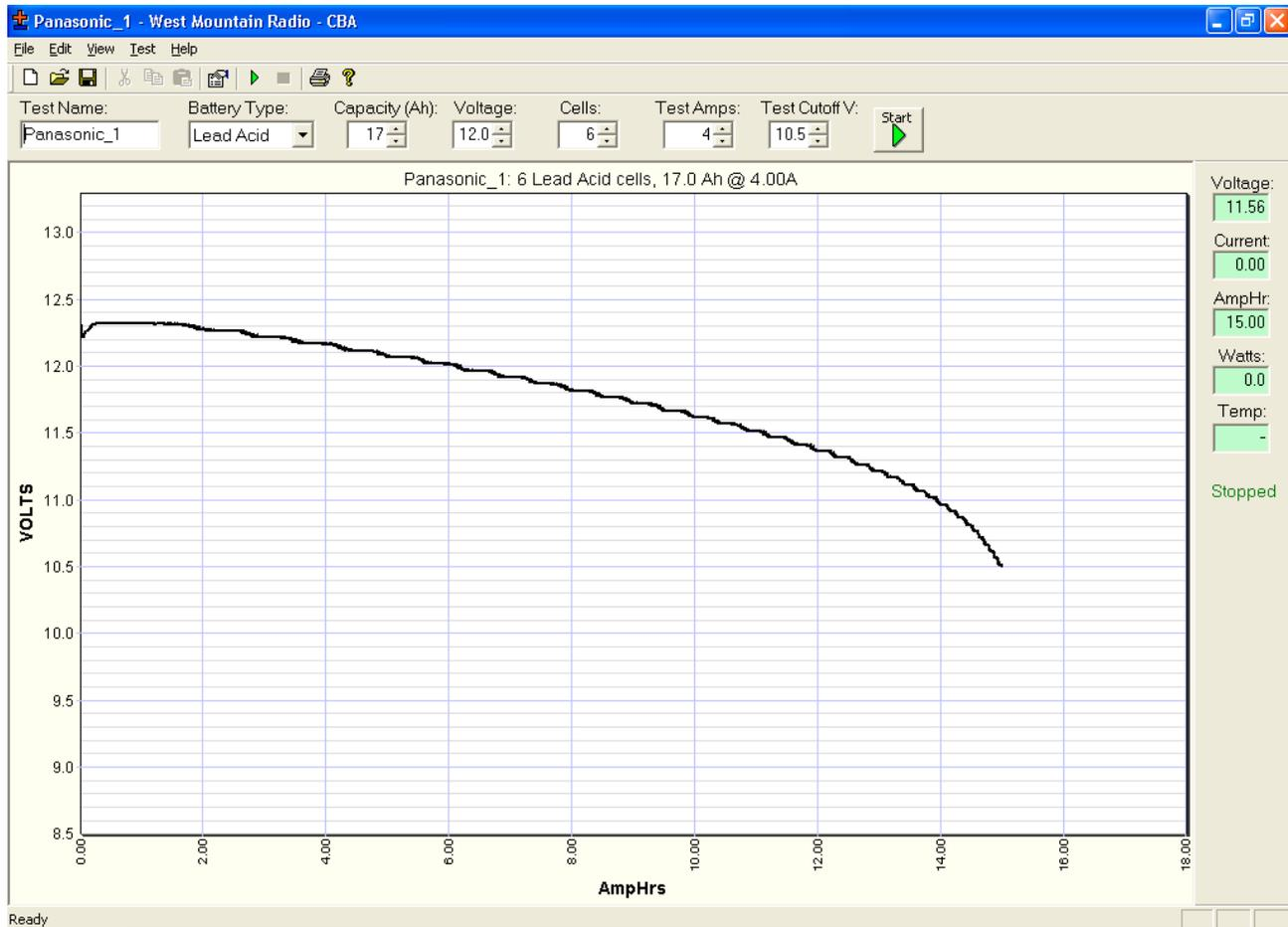
As you can see here, when discharged to simulate a 4A e-bus load, the ol' beast trudged along for 15 a.h. worth of output. Given that it's rated for 17 a.h. under a 20 hour rate, it seems that this battery might still be performing at or near new specifications for capacity in spite of disappointing value of source impedance.
