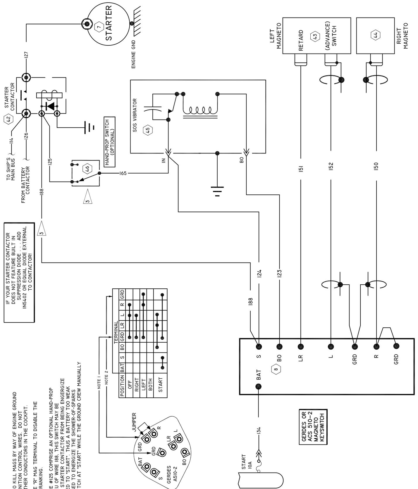
A SPECIAL IMPLEMENTATION OF S.O.S. IGNITION FOUND ON SOME MOONEY AIRCRAFT THAT FEATURES A "HAND PROP SWITCH". THE STARTER CONTACTOR IS DISABLED SO THAT THE SOS SYSTEM CAN BE INDEPENDENTLY ENERGIZED BY HOLDING THE KEY IN THE "START" WHILE THE PROP IS SIMPLY PULLED THROUGH T.D.C. AS SOON AS THE RETARD POINTS OPEN, THE ENGINE COMES TO LIFE.
