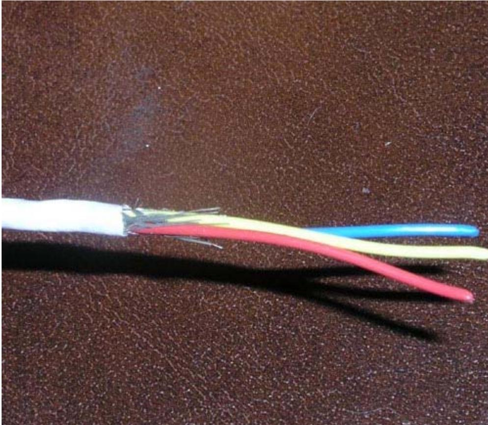
You wind the shield remnants tightly around the wires like this . . . keep the diameter small.
