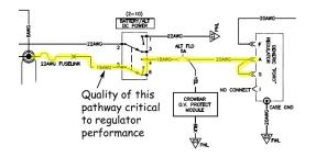
The 'ford' regulator will be just fine if you take steps to maintain integrity of the v-sense/field-supply path. Make all terminations with gas-tight devices installed with compatible tools.
