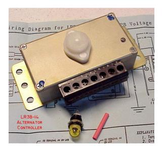
The only regulators I'm aware of with separate sense path are the B&C LR/LS series devices. From the getgo, B&C decided that any such product offered would be an ALTERNATOR CONTROLLER consisting of a remote sense regulator, built in over voltage management and active notification of low voltage.
