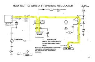
I've only designed one 3-terminal regulator per specs supplied by the customer . . . all subsequent designs featured at least a positive voltage sense; sometimes both positive and negative sense paths. This provided for much improved performance over the lifetime of the regulator.
