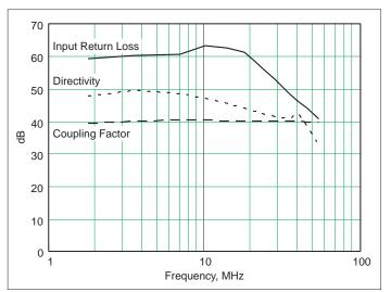
Figure 8 - Measured Bruene Bridge Characteristics (Including log amps)
