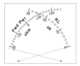
Figure 11 - Dual Movement Meter Scales, shows power off needle resting positions
