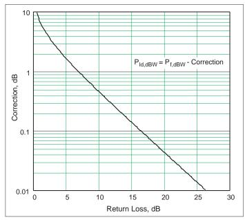
Figure 3 - Load Power Correction Using Measured Forward Power and Return Loss
