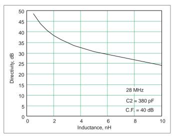
Figure 7 - Bruene Bridge Directivity Sensitivity to Lead Inductance
