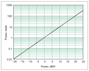
Figure 4 - Convert Power in dBW to watts
