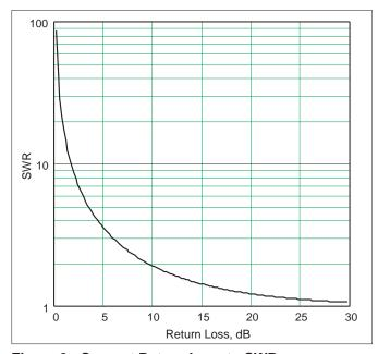
Figure 2 - Convert Return Loss to SWR
