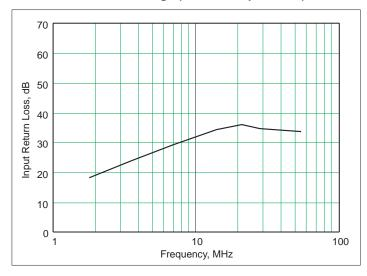
Figure 6 - Measured Tandem Match Coupler Input Return Loss
