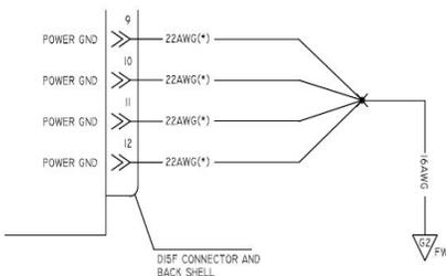
There are some instances where your greater-than-5A current path plugs into a connector where there are no ballasting resistors associated with the paralleled pins. No problem, just put full 12" pigtailed on the harness side.
