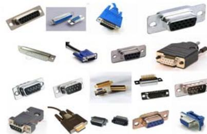
There are hundreds of configurations offered with pin counts ranging from 9 to 50 for 20AWG wire. Specialized versions are also offered with fat-wire pins and pins designed to carry coaxial cable feeders through the connector. Hi-Density and Micro-D versions offer high-density 22AWG pins still greater wire counts in a small space.
