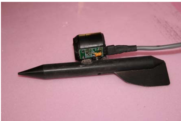
AOA Vane and Mount with Hall Sensor
