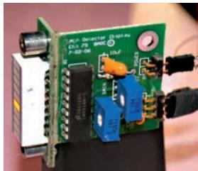
**AOA display boards require minimal panel space but should be mounted high on the panel to stay within your peripheral field of vision while looking outside.**
