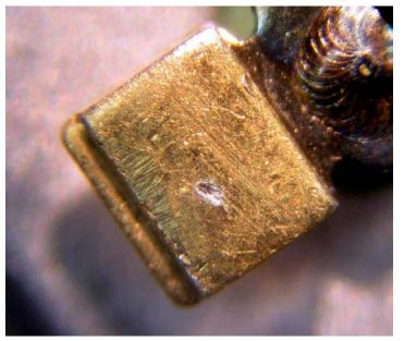
absolute magnitude of metal transfer is not a major clue as to root cause. Clearly these relays can continue to function within specified limits in spite of significant metal transfer. As a part of their QPL requirements, Deutch routinely demonstrates that the relay meets operating requirements in spite metal transfer several times more severe than troublesome relays removed from the roll trim system.
