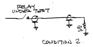
**Condition 2** A second test article was run with the RFI filter capacitor removed.
