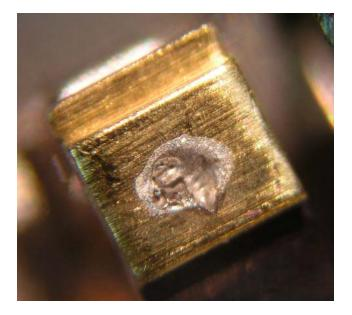
This view shows footprint of the crater for moving contact of Section A. In spite of this remarkable metal transfer, the contact was still operating freely after 500K cycles.
