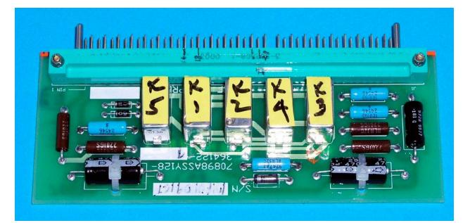
Field failures of roll trim relays are attributable to low\_force sticking of contacts in spite of the fact that electrical stresses on the relays are well inside the ratings envelope for the device.
