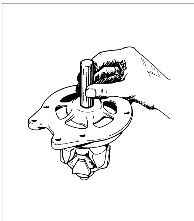
Figure 24-35. Installation of Drive End Head
