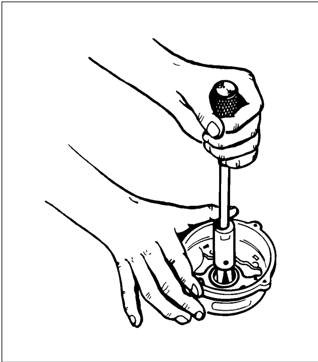
Figure 24-29. Removal of Slip Ring
