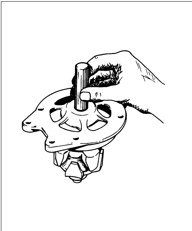
Figure 24-10. Installation of Bearing
