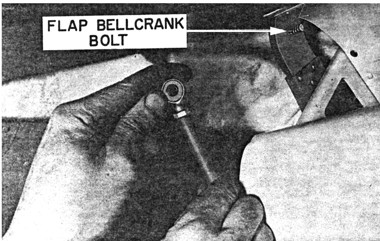
Figure 5-15. Adjusting Flap Control Rod End Bearing
