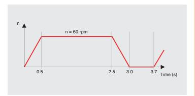
The inertia of load  $J_{\rm L}$  to be accelerated is 130 000 gcm². The constant friction torque is 300 mNm. The motor is to be driven with the linear 4-Q servo amplifier from maxon (LSC). The power supply delivers max. 5 A and 24 V.
