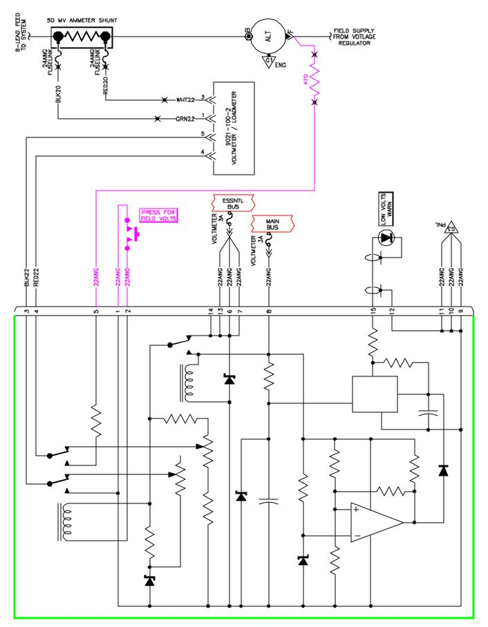
**3.1.7** Momentarily depress the alternator system diagnostic button. The voltmeter should read less than 14.0 volts on the instrument (12 volts in real life). As engine RPMs increase, field voltage should go down. Daytime cruising flight may require field excitation of less than 3 volts (11 volts indicated on the instrument)
