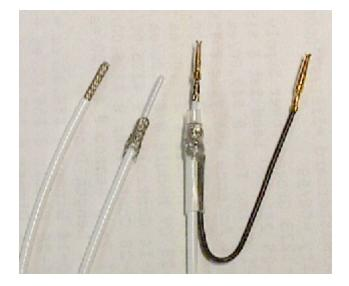
**2.2.2** Attaching the shielded wire to the D-sub connector takes a little "maneuvering". Strip 3/8" of outer jacket from the shielded wire and push the shield braid back over the top of the outer jacket.
