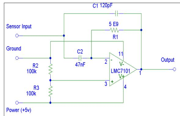
Figure 2. Charge Preamplifier
