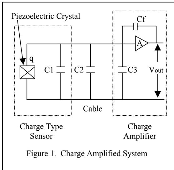
The output voltage is dependent on the ratio of the input charge to the feedback capacitance as shown in Equation 1 below. Note that the capacitance due to the sensor, cable, and amplifier (C1, C2, C3) do not affect the system sensitivity.
