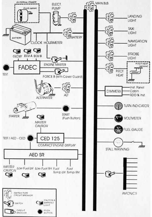
Figure 1-4b Basic Wiring of the Electrical System with Switch Alternator
