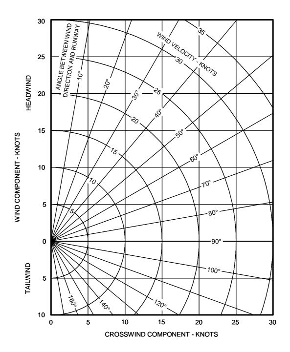
Figure 5-4. Wind Components
