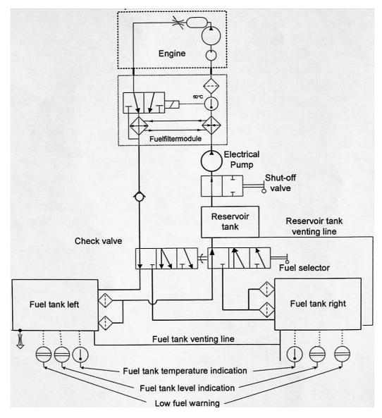
Figurel 1-3b Scheme of the Fuel System (Left, Right, Both)
