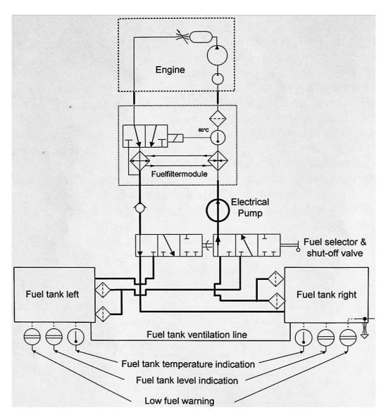
Figure 1-3a Scheme of the Fuel System (Left, Right)
