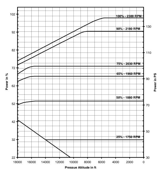
Figure 5-9 Engine Power Over Altitude
