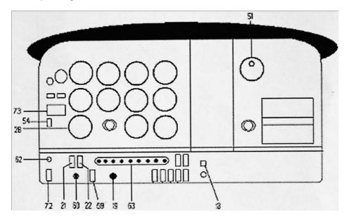
Figure 1-2a Example of Instrument panel with TAE 125 installation (with circuit breaker Alternator)
