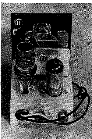
Front, rear, and bottom views of a compact one-tube receiver that you can take along almost anywhere. Power to operate the tiny set is supplied by a 1.5-volt flash-light cell and a midget 45-volt battery
