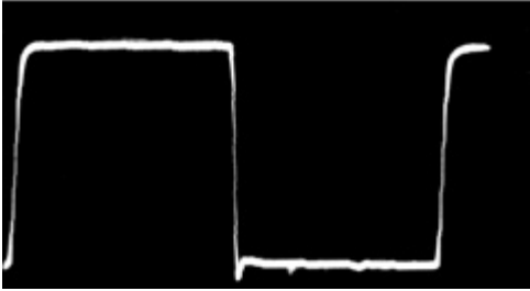
3-8B TDR pulse with no significant reflection.
