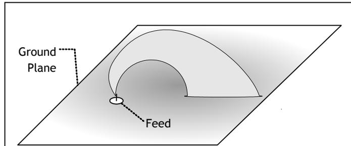
Figure 3: Scimitar antenna of Turner et al.
