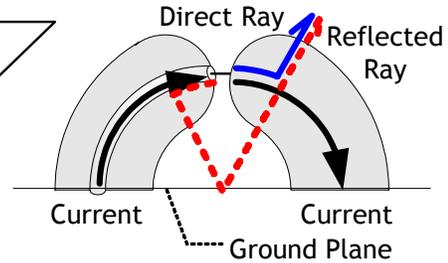
Figure 7: Current and radiation from a center fed monoloop.
