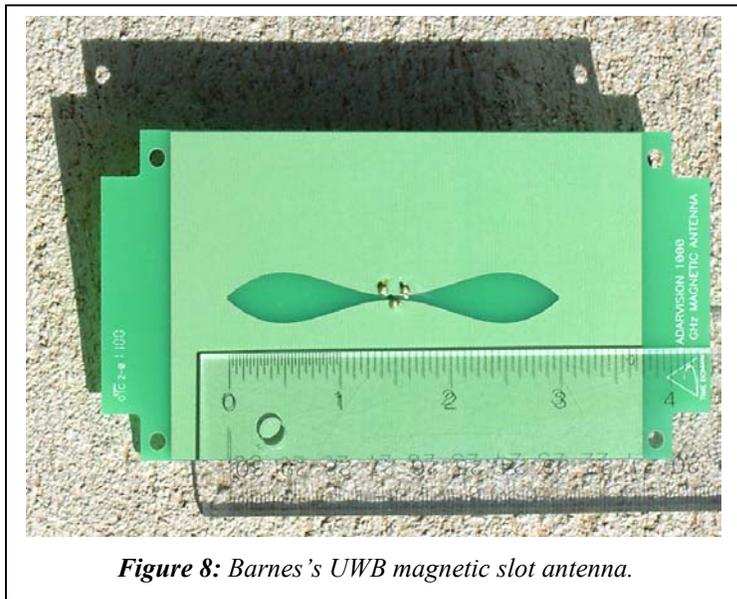
Figure 8: Barnes's UWB magnetic slot antenna.
