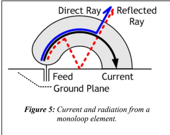
Figure 5: Current and radiation from a monoloop element.
