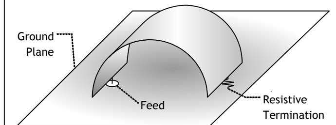
*Figure 2: Balanced-dipole antenna of Farr et al*
