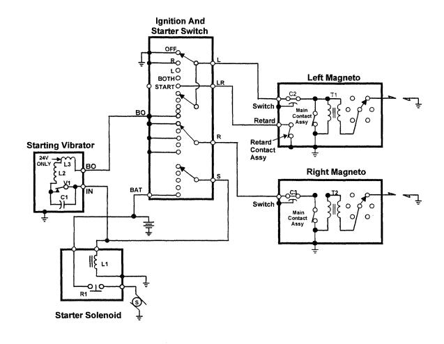
Figure 3-1 Typical Ignition System With Starting Vibrator
