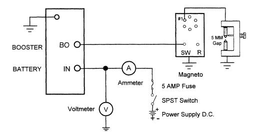
Figure 4-1 Test Setup For Starting Vibrator
