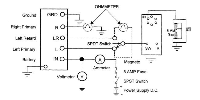
Figure 4-2 Test Setup For Vibrator With Relay
