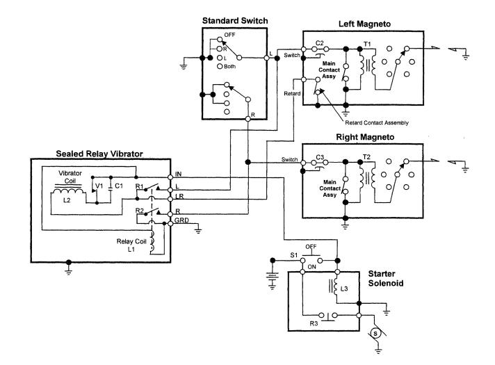
Figure 3-2 Typical Ignition System With Starting Vibrator With Relay
