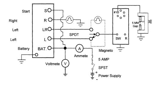
Figure 4-3 Test Setup For Starting Vibrator With Relay And Delay
