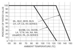
Figure 5. Current, Energy, Power Derating v/s Temperature.
