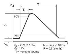
Figure 3. Load Dump Transient
