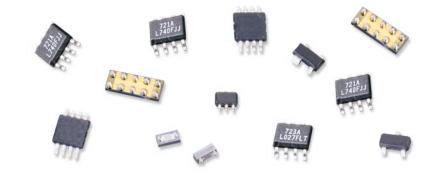
clamp device returns to its off state. There are two main product types within the rail clamp technology. This includes a high voltage (30V) SP72x family and lower voltage (5V) SP05x family.
