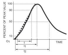
Figure 4. Peak Pulse Current Test Waveform
