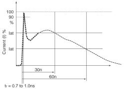
Figure 2. ESD Test Waveform
