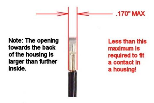
YOU WILL NOT BE ABLE TO INSERT THE CONTACTS INTO THE HOUSINGS IF THEY ARE TOO WIDE AFTER SOLDERING OR CRIMPING!
