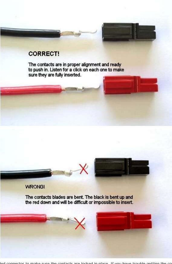
Tug slightly on the assembled connector to make sure the contacts are locked in place. If you have trouble getting the contact to lock in to the housing you may have squashed the contact wider deformed it some how. Look at the side profile of the contacts before and after crimping, you may have to bend it back straight before inserting it in to the housing.
