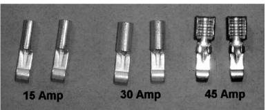
• 30 amp contacts can be used with #12-16 AWG wire. (It is possible to use up to #10 wire in a 30 amp contact even though they are made for 12 to 14 gauge. The #10 will need to be cut cleanly and neatly twist it to get all of the strands inside. For #18 AWG or smaller the wire will have to be doubled or tripled over to fill the contact for a good crimp.)
