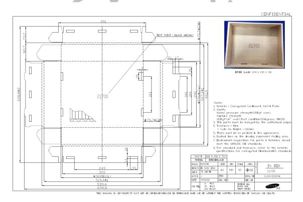
Fig. 2-2. Inner box package drawing.
