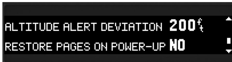
Figure 6-17 Altitude Alert Deviation and Restore Page
