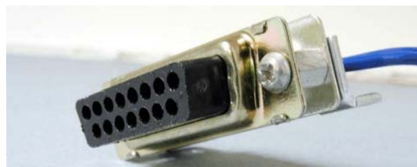
Figure 18-16. DIY D-Sub Ground Block, Wiring Side
