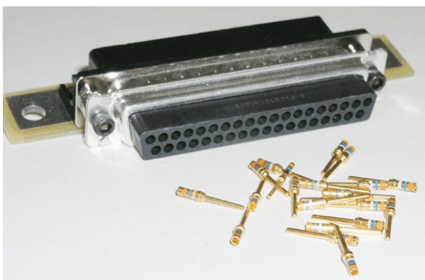
Figure 18-14. Manufactured D-Sub Ground Block
