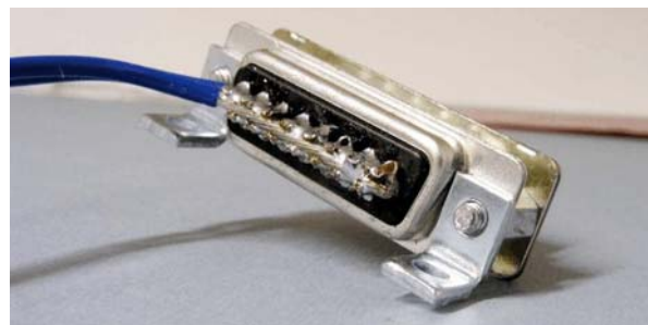
Figure 18-15. DIY D-Sub Ground Block, Rear View
